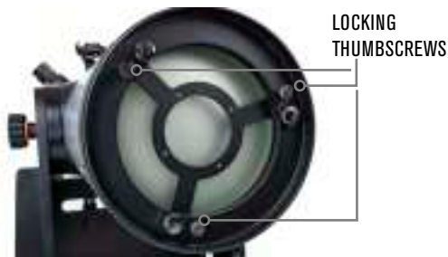
Figure 21: For the 10" Dob, there are three spring-loaded collimation thumbscrews that adjust the tilt of the primary mirror. The other three thumbscrews lock the mirror in place once tilt adjustments are completed.
