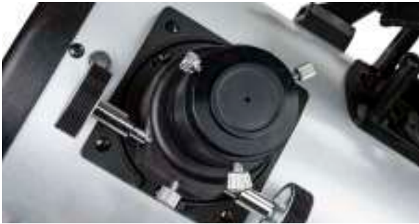
Figure 15: To check the alignment of the mirrors, use the included collimation cap in the focuser.
